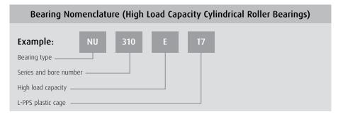
This screw compressor specification includes high-capacity design, and L-PPS « T7 » cage. Range: From 20 to 100 mm bore (NU204ET7 to NU2320ET7)
