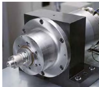
NSK Spindle that achieved 4 million d_m/n using ceramic ball bearings
