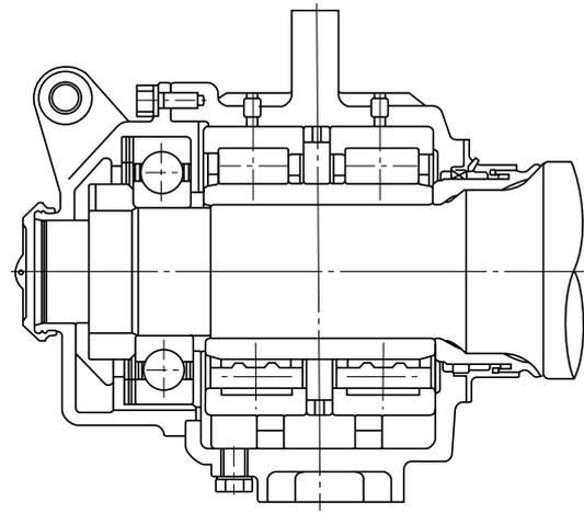
**Axle Box with Deep Groove Ball Bearing and
