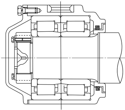
**Axle Box with Roller-Guiding Ribs to Sustain Axial Loads
