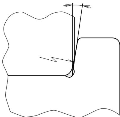
Fig. 7-1 The design of rib and roller end
