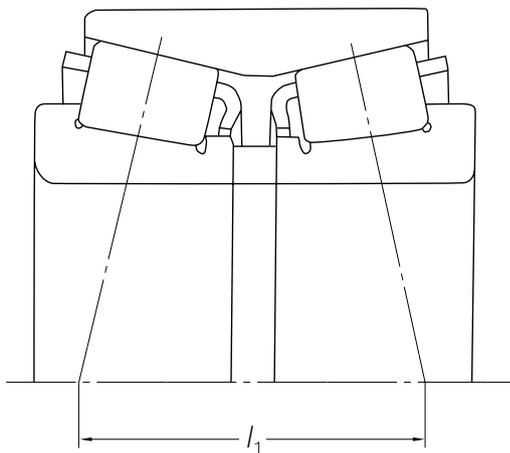
**Fig. 5-1 Back-to-Back Arrangement**
